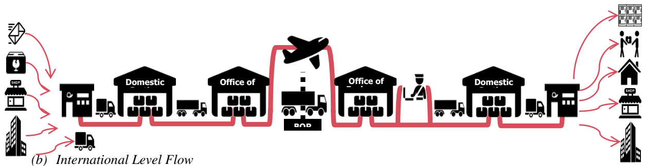
Figure 3: Acceptance, sorting, air transportation, sorting and delivering of mail items Int'l system
